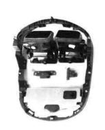
3 Remove all the components from the original facia plate as shown in the picture:
