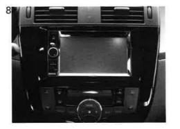
8 Connect all the cables, check the correct operation and fix the facia plate. In the picture it is shown the final result.
