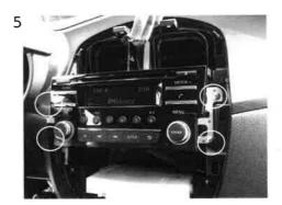
5 Remove the original radio from its position by unscrewing the screws.
