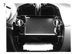
7 Place and fix with the supplied screws the aftermarket head-unit to the dashboard.
